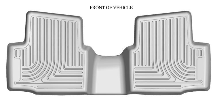
TO EASE INSTALLATION OF YOUR CRUZE SECOND SEAT LINER, MOVE THE FRONT SEATS TO THEIR MOST FORWARD POSITIONS. WITH THIS DONE, INSERT THE LINER IN YOUR VEHICLE. WITH THE LINER IN PLACE, REPOSITION THE FRONT SEATS AS DESIRED.
