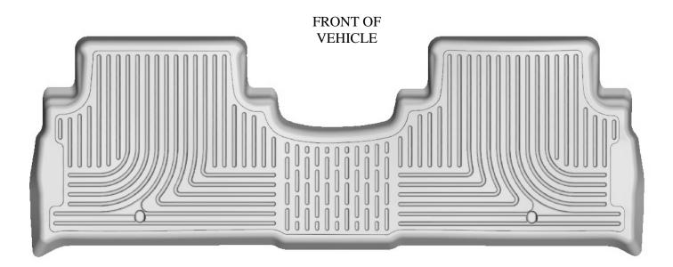
TO EASE INSTALLATION OF YOUR 2<sup>nd</sup> SEAT SORENTO FLOOR LINER, FIRST MOVE THE FRONT SEATS TO THEIR MOST FORWARD POSITIONS. WITH THIS DONE, INSERT LINER IN VEHICLE THEN REPOSITION THE FRONT SEATS AS DESIRED.
