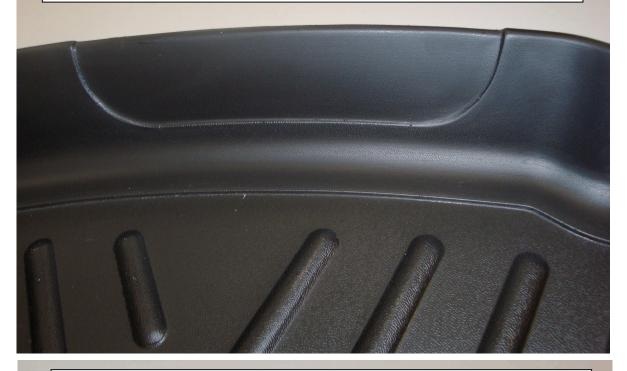
PHOTO SHOWING PART #42051 TRIMMED TO ALLOW ACCESS TO CARGO HOOK AND CARGO NET RETAINER.
