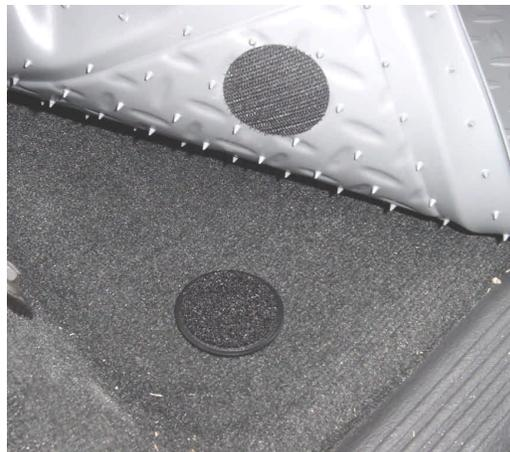
PHOTO 3. ANCHOR SCREW SHOWN INSTALLED IN CARPET ALIGNED BELOW HOOK PAD.
