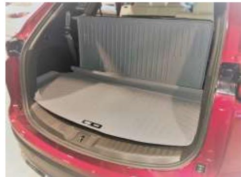
6. The liner at this point is fully installed and is ready to use. If the liner needs to be removed, grab the rectangular Velcro patches and hold them firmly in place as you pull the liner from the seat. This Velcro piece is intended to stay attached to the seat back and cargo floor to reduce wear from the liner being installed and reinstalled for cleaning.
