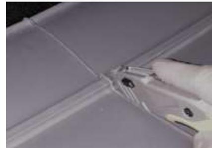
3. If your seats fold manually you may want to trim out the two seat back release access openings as shown. To trim, use the recessed trough around the inside bottom of the opening. A utility knife works well for trimming. If you have power operated 3<sup>rd</sup> row seat backs this step is not needed.
