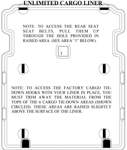
TO ACCESS THE FACTORY CHILD SEAT SAFETY RESTRAINT ANCHORS, TRIM AWAY THE MATERIAL FROM THE TOPS OF THE TWO (2) RAISED AREAS (SHOWN ABOVE DARKENED).
