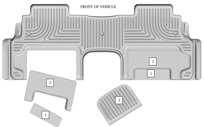
YOUR VEHICLE IS EQUIPPED WITH  $2^{\rm ND}$  ROW BUCKET SEATS THAT CAN BE ADJUSTED TO MULTIPLE CONFIGURATIONS. PART #1921 IS DESIGNED TO ACCOMMODATE THESE POSITIONS. WITH YOUR SECOND ROW SEATS POSITIONED FOR MAXIMUM  $2^{\rm ND}$  ROW PASSENGER LEG ROOM, YOUR LINER WILL FIT AS BOXED. IF YOU WISH TO REPOSITION YOUR  $2^{\rm ND}$  ROW SEATS FOR MAXIMUM  $3^{\rm RD}$  SEAT PASSENGER LEG ROOM, TRIM AWAY THE MATERIAL FROM THE TWO RAISED AREAS LOCATED ALONG THE BACK WALL OF YOUR LINER (SEE AREAS
