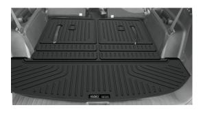
5. The first time the rear seat backs are moved to the upright position, move the seats slowly taking care to insure the accordion section of the liner folds outward as shown. This may need to be assisted from the backside.
